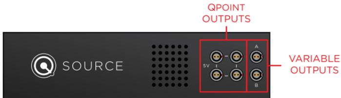
Outputs “A” and “B” are controlled by the corresponding switches on the bottom of the QSOURCE. Output “A” supplies 24, 19, or 12 VDC, while output “B” supplies 19, 12, or 9 VDC. Select the correct voltage necessary for your device before connecting any devices or powering on the QSOURCE.
