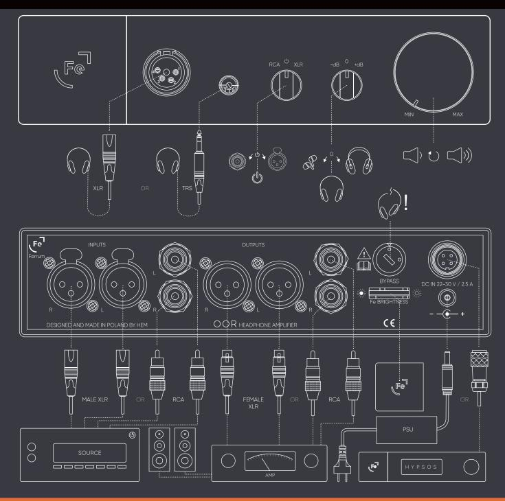
Connect all the cables before switching on the OOR.
