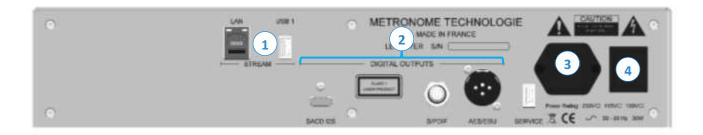
1 : Ethernet and USB Inputs (streaming option
