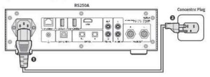
∆ Caution: When disconnecting the power cord, always disconnect the outlet first.
