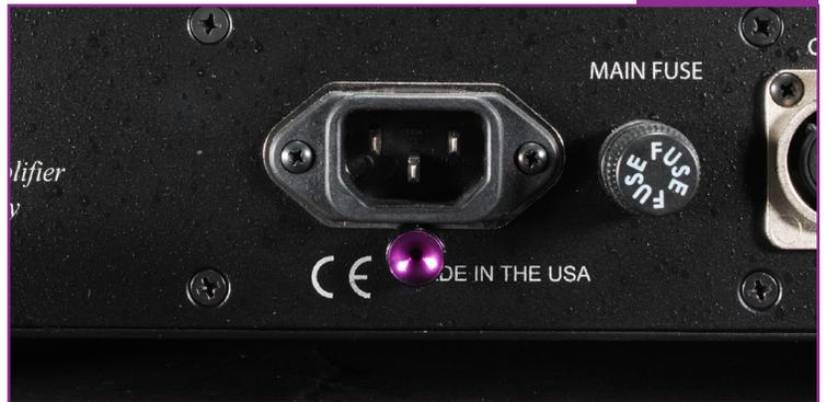
• IEC Ground Placement: Apply a small amount of \*white tack or glue dot to the bottom of the GCT and affix near the IEC ground pin.
