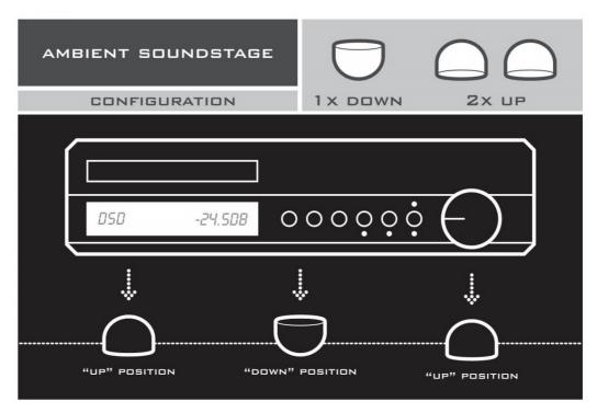
When two Mig 2.0s are placed "round side up" and one MiG 2.0 is placed "round side down" under a component, as illustrated in the above diagram, you hear a more ambient soundscape that is especially pleasing when room acoustics are somewhat "live" or undampened. You may also prefer this combination if you like a slightly more liquid presentation, or if you often listen to large orchestral works.
